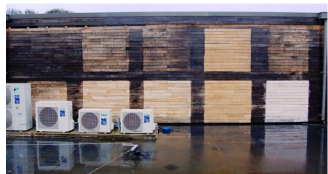
Figure 9 Test areas on sweet chestnut 14 months after cleaning, showing differential levels of re-colonization according to treatment
